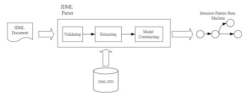
Fig. 2. The concept of IDML parser.
