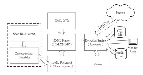
Fig. 5. An IDML-based intrusion detection experimental system.
